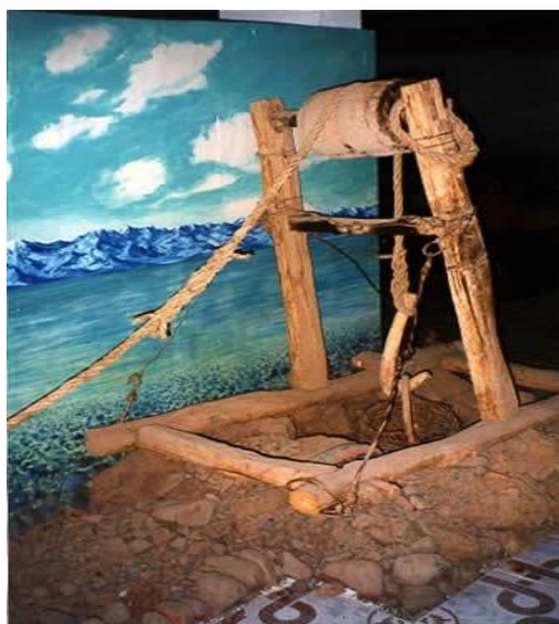
Figure 7: Windlass used to build qanats. http://www.waterhistory.org/histories/qanats/
