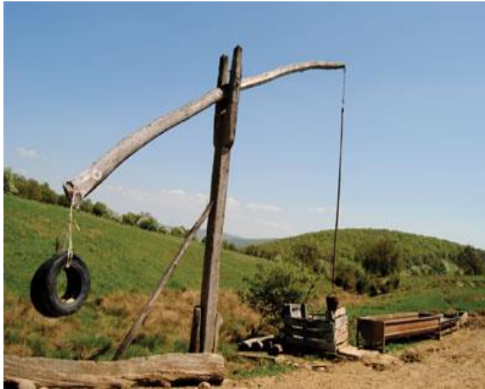
Figure 5: Shaduf, a type of bucket and pulley invented in ancient Sumer. http://www.groundwatercanada.com/index.php?option=com_content&task=view&id=1810&Itemid=134
